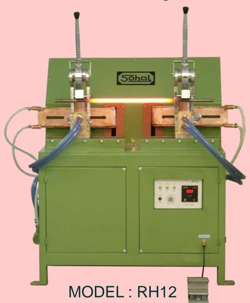
Resistance heating machines are best suitable for rod heating in U-bolt manufacturing industry. These machines have less running cost compared to oil furnaces. These are simple to operate and durable. The 50 KVA machine is designed for flat type U-bolt make. The heating temperature is set by electronics power control thyristors and timer.
